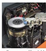
Operators will quickly notice the solid feeling and responsiveness of the dynamic hydraulic brake. Here the Toyota design minimizes the mechanical loss that takes place when the brake pedal is pressed. Not only does this design provide enhanced responsiveness, it also reduces the amount of effort needed to operate the brake.
