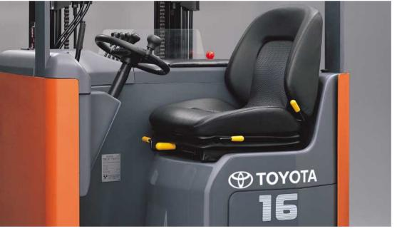
Toyota knows that operability can be as important as basic load handling performance when it comes to boosting productivity. The voltage and amperage hybrid control function on this series provides what Toyota calls proportional response -- a smooth, progressive and predictable movement of the reach truck and its components that is proportional to the amount the controls are
