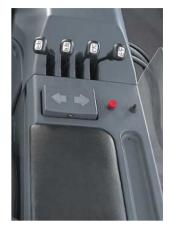
The efficient layout of the operating control levers and direction switch are another example of Toyota practicality. Here minimal operator effort is needed to safely and productively use the controls.
